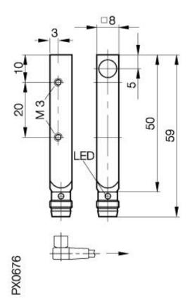
Inductive Sensors BES 516-300-S 166-S 49 8 x 8 x 59 normally-open Sn=1,5mm shielded
